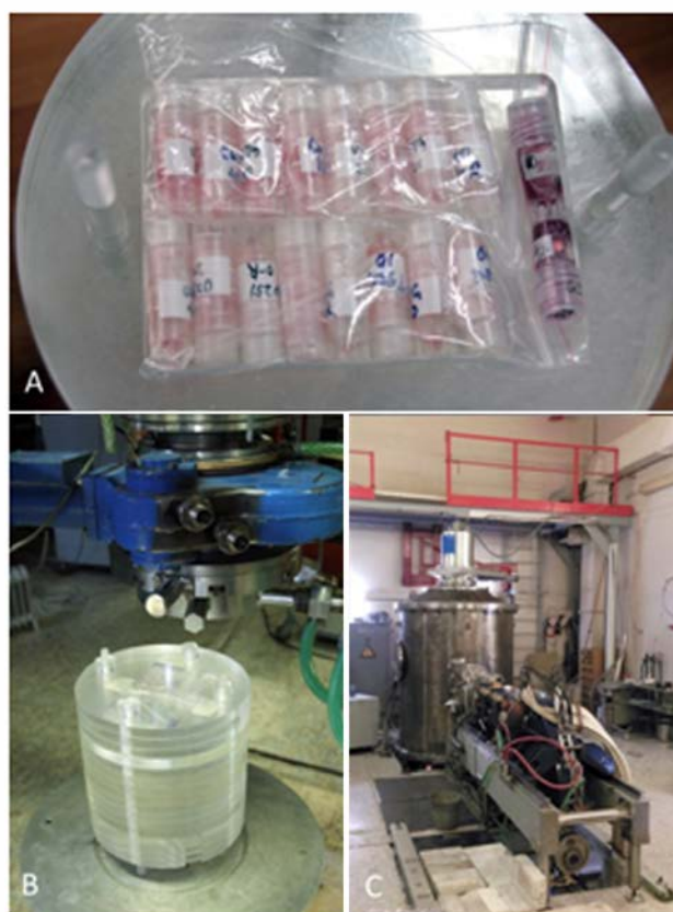
FIGURE 2. Process of specimen irradiation. U251MG cells were placed in plastic vials (A) in a phantom made of organic glass under the lithium target (B) of the tandem accelerator with vacuum insulation (C)
